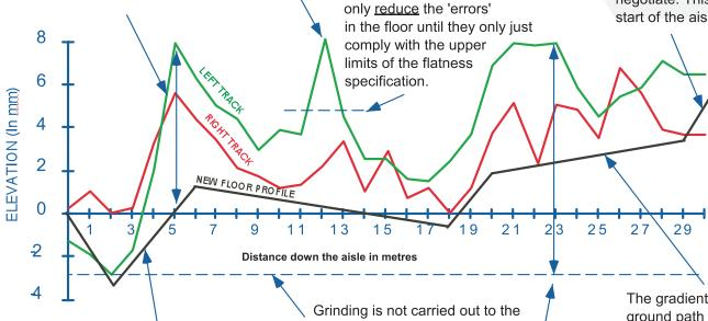
This line represents the new profile of both the left and right wheel tracks, (or the whole aisle width if required), after the Laser Grinding process is completed. level of the lowest point of the existing floor, as this would mean unnecessarily deep cuts. (In this case over 10mm deep to the right track at 23 metres along the aisle)
